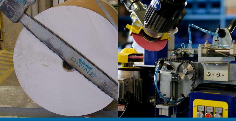
For paper rolls cutting we use special, carbide tipped chain DURACUT 15/3. 8mm long cutting edge and scraper type for smooth and even surface after cutting. Guide bars are available with one or both sides stellite plating, ensuring the longest endurance. All cutting unit parts are produced in PRINZ, Austria.
