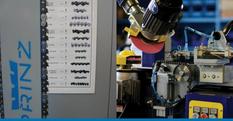
Cross-cut saws, based on the type of cut material, manner of cut and intensity of servicing, can be equipped with scraper saw chains for cutting packages, chipper saw chains for roundwood or carbide tipped saw chains for hard, dirty or frozen wood. Guide bar are available in high frequency hardened version or with stellite layer on one or both sides. All spare parts produced by PRINZ.
