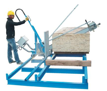
**TWIN-L** mobile saw with positioning frame
