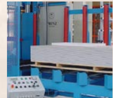
Cutting gypsum plates
