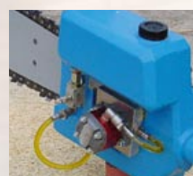
Lubricating the cutting edge
