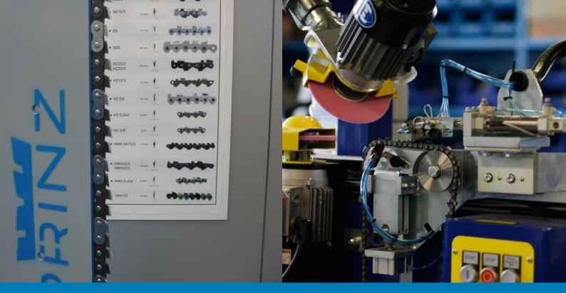
Cross-cut saws, based on the type of cut material, manner of cut and intensity of servicing, can be equipped with scraper SZ, chipper HZ or carbide tipped HMH saw chains. Guide bars are available as high frequency hardened version or with stellite layer on one or both sides.
