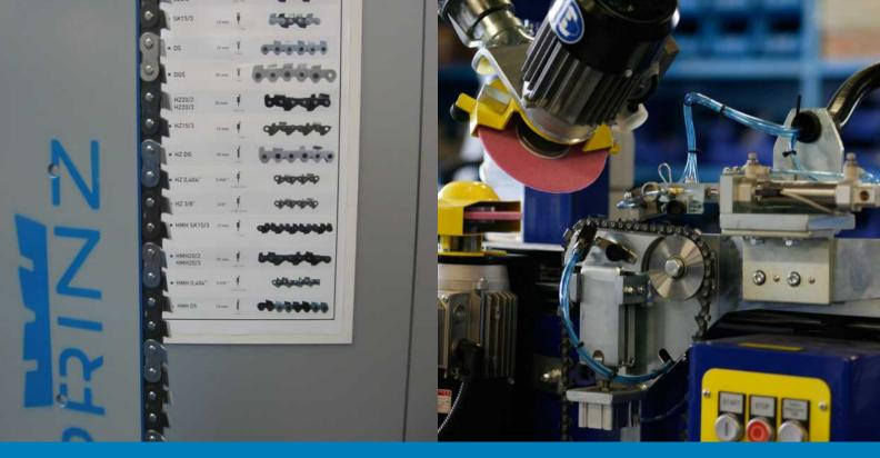
Cross-cut saws, based on the type of cut material, manner of cut and intensity of servicing, can be equipped with scrapper SZ, chipper HZ or carbide tipped HMH saw chains. Guide bars are available as high frequency hardened version or with stellite layer on one or both sides.
